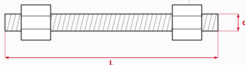
Stud bolt with two heavy hex nuts; L excludes the point height at each end
